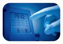
A touch screen allows users to select preset protocols or design new ones. The screen can be controlled remotely using an Internet connection.
