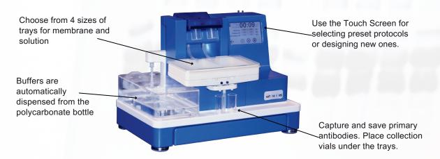
Traditional western blot analysis is a time-consuming process. **NeoBlot Auto™ Mini** changes everything by automating the fluid changes and timing associated with blocking, washing and antibody incubation. There's no more need to watch over the western blot procedure. With BlotCycler Mini, simply set up your protocol, and walk away!
